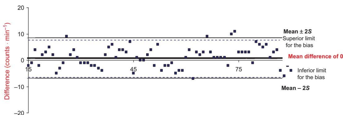
Figure 3. Difference in accelerometer counts between the two devices in moderate intensity.
