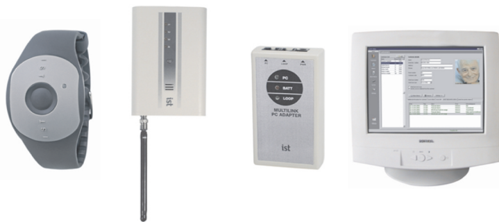
Figure 1. The IST Vivago® WristCare system for activity level monitoring (3001 wrist unit, base unit, IST bus adapter and Vista software)
