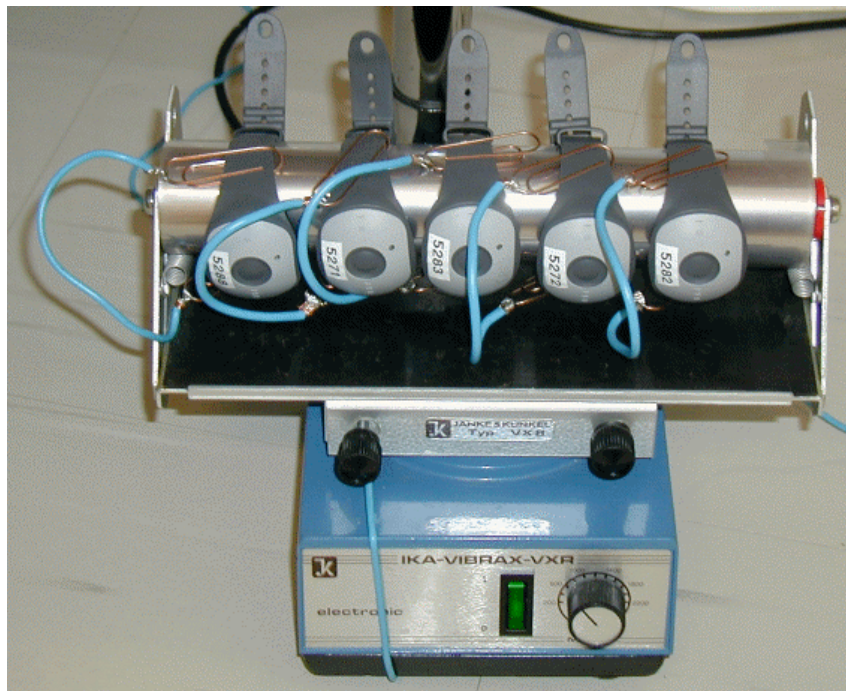
The shaker used for simulating wrist movements, shown with several WristCare units on it. The 'wrist simulator' cables are clearly visible too.
